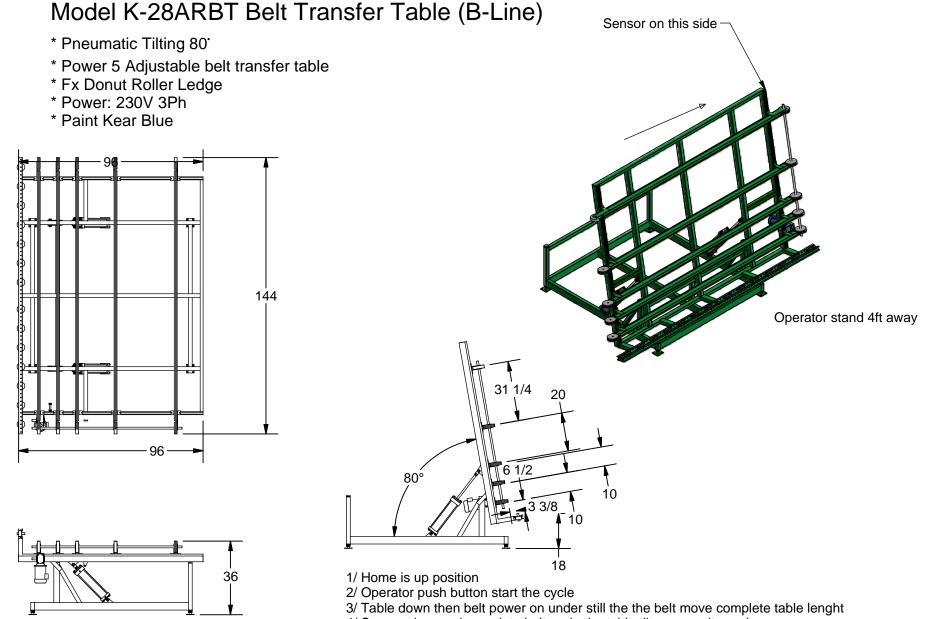
4/ Sensor clear and complete belt cycle the table tilt up complte cycle
