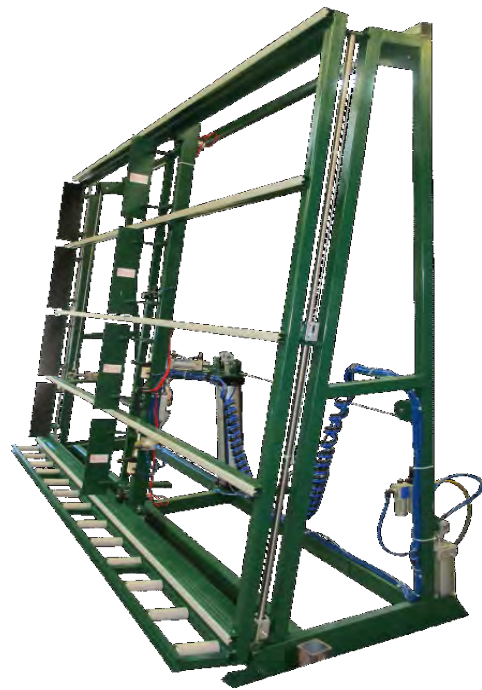
K-34RT Pneumatic Clamp, Lift, Tilt Square & Glazing Rack
