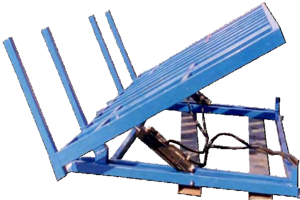
K-2HDC Hydraulic Tilt Aluminium Windows & Curtain Wall Packaging Table
