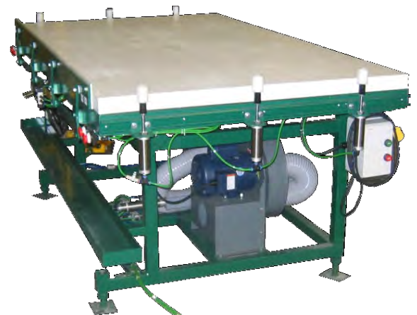
K-37GT Grill Assembly Table with Pneumatic Tilt and Pop up Ledge
