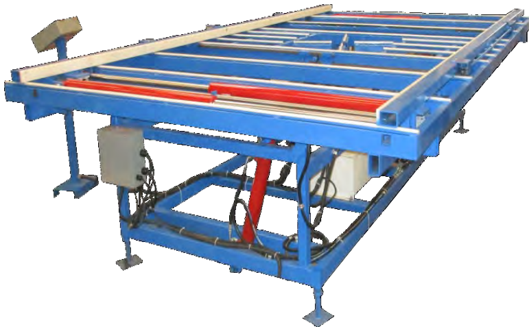
K-28PP-H Hydraulic Tilt, Clamp Table
