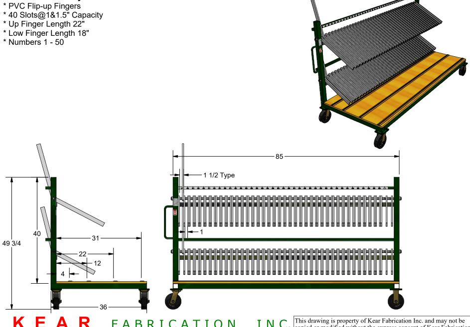
FABRICATION 27 Vanley Crescent, North York, ON, M3J 2B7 - Tel: (416) 398-8666 - Fax: (416) 398-9666 This drawing is property of Kear Fabrication Inc. and may not be copied or modified without the express consent of Kear Fabrication Inc. All dimensions are in inches and are accurate to 1/16". Angles are accurate to 1/2°. Report all changes and/or errors to the Kear Fabrication Inc. Engineering Department.
